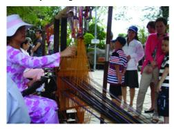
What caught my eye was the patterningsystem. Both looms had a ground warp woven as plain weave using two shafts, the warp and weft were the same, a fine cotton. Each loom had two pedals to weave the ground cloth, each connected to alternate ground warp threads.
