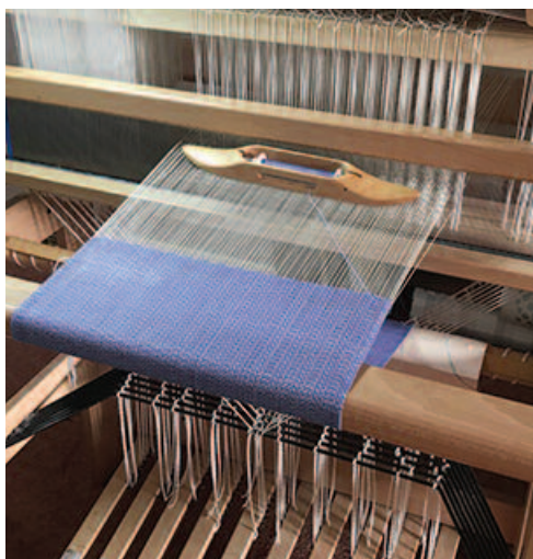
Jacqueline H - (above) My 8 shaft Louët David dressed with a 2/25nm silk warp and 2/16nm Bamboo in Periwinkle. The pattern draft is from Strickler No. 396: (left) deflected doubleweave on the loom.
