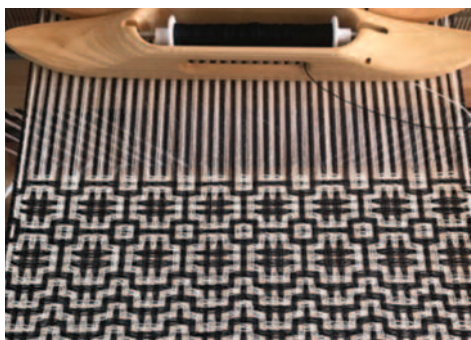
Jacqueline H - (above) My 8 shaft Louët David dressed with a 2/25nm silk warp and 2/16nm Bamboo in Periwinkle. The pattern draft is from Strickler No. 396: (left) deflected doubleweave on the loom.
